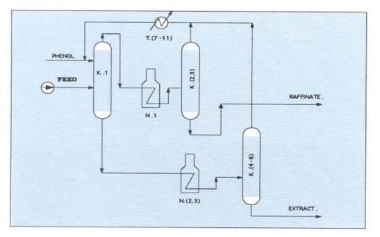
Figure (17): Phenol Extracting Unit.
