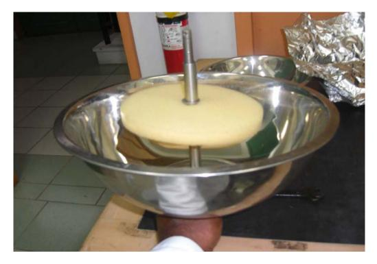
Figure (25): Air sampler containing the PUF filter
