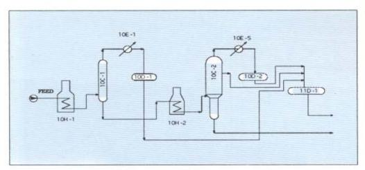
Figure (13): Skimmed Crude Two Stages Distillation Unit.
