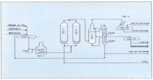
Figure (14): Delayed Coking Unit.
