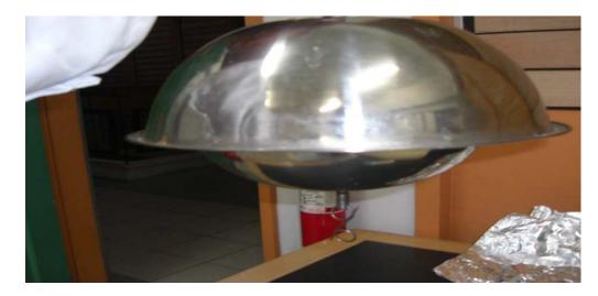
Figure (26): The PAS sampler is ready for deployment onto monitoring site
