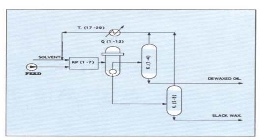
Figure (18): Dewaxing Unit.
