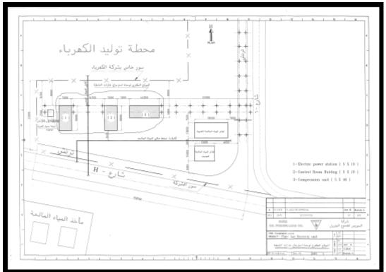
Figure (23): Proposed Position for the flare gar recovery Unit (Large Scale).
