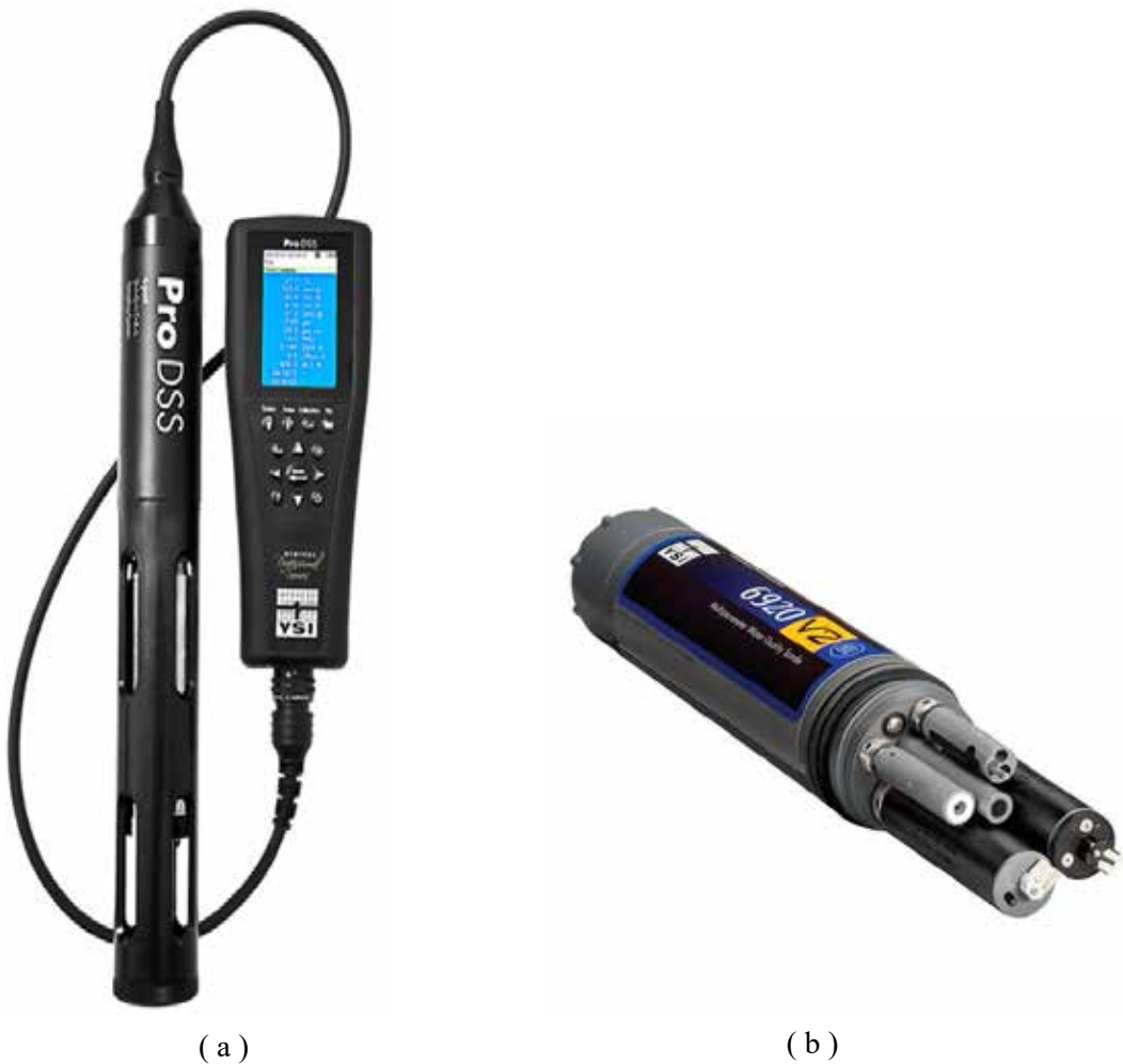
Figure 4.3 Examples of the types of multi-parameter probes (a) YSI PRODSS Multi-parameter probe which can monitor up to 4 parameters, it has a hand held device attached which displays the readings. This model can be equipped with a cable up to 100m depth and a built in GPS; (b) YSI 6920 series sonde, which can be attached to a handheld data logger, similar to probe shown above. The sondes offer the potential to monitor more parameters and can be left in-situ for continuous monitoring.
